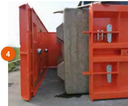
4 When the mould is opened, the magnet remains in the mould
