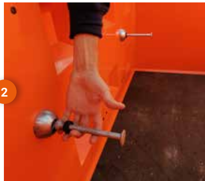
2 Place the rubber around the anchor, place the anchor in the magnet
