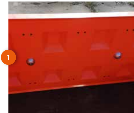
1 Place the magnet in the center of the mould
